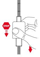
holder's self-locking mechanism is triggered.
