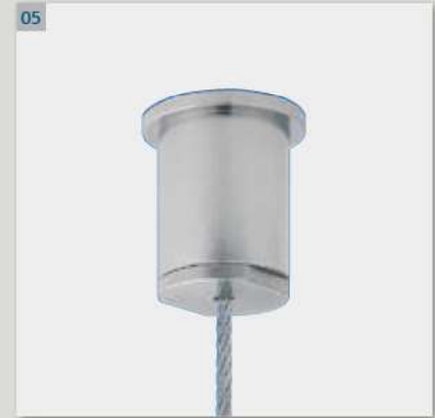
05 Ceiling attachment M13x1; M6i short and screw cap M13x1 with bore 2.4 mm SW 14
