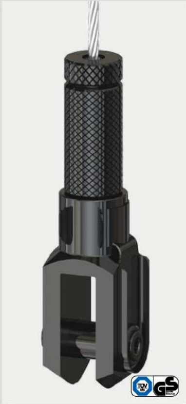
01 Holder type 30 SV m.R. with fork 10x20 and safety-bolt, black zinc-plated
