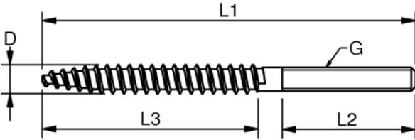
The dual thread pin allows direct installation into wood and if combined with the correct raw plug it is attachable to almost any wall. Ideal for inside thread solutions.
