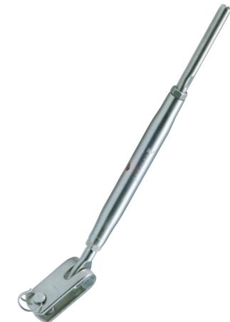
Blue Wave rigging screws bodies feature thread size, "easy use" marking for left and right threaded side and adjustment hole. From M20 upwards the bodies are available with chrome bronze threaded inserts and spanner flat on body, for smooth adjustment.
