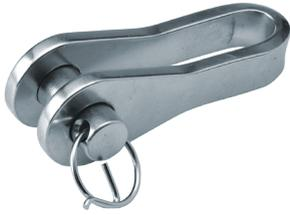
For lengthening the wire, or adding flexibility to installations, the toggles can be applied. Where a structure is subjected to stress the use of a toggle is essential as it can minimise the fatigue risk.
