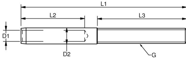
Blue Wave's small thread terminals are for lighter architectural fixing of wires. The focus of the design is the size. Overall dimensions have thus been reduced to a minimum. The small fittings are suitable for hand crimping with Blue Wave Arctool1ACC & Arctool8, see page 61, or roll swaged using a standard machine and smaller die.
