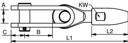
In addition to the Lloyds approved swageless system, the swageless cone terminal for 1x19 wire construction enables safe and reliable wire attachment up till Ø 26 mm diameter.
