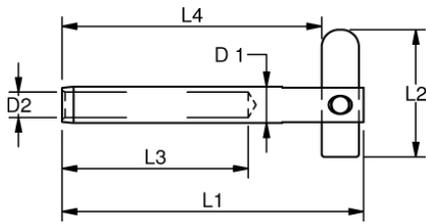
The dropnose terminal is e.g. perfect for tube handrails with vertical wire suspensions. Almost the easiest mounting imaginable - after being attached to the wire, drill a hole and stick through the drop nose end of the terminal and let it drop!
