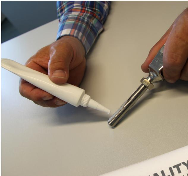
The Blue Wave Lubricant is used on the threads improving the performance. Whenever stainless steel threaded parts are screwed together it is always strongly recommended to lubricate the threads first, as this prevents the threads from jamming!
