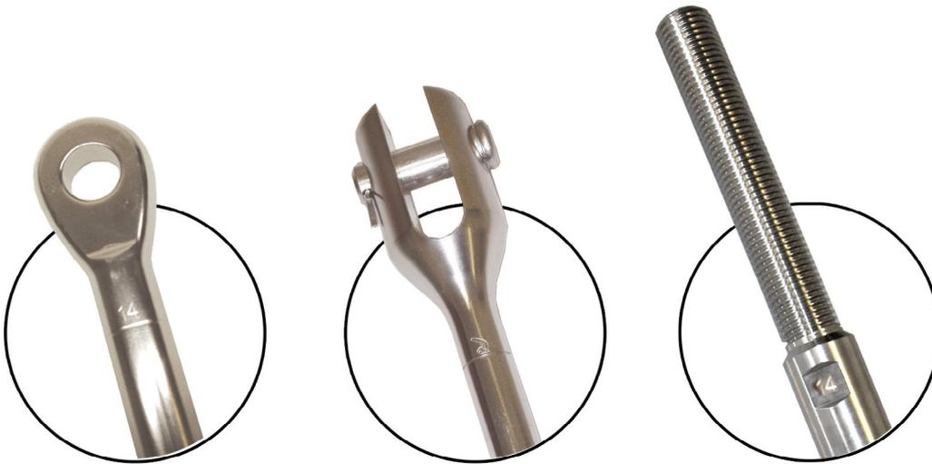
Where markings are not possible e.g. on the small terminals, the wire hole depth must be measured before swaging, not only to find the point to start the swaging, but also to get the right length of the final wire including the fittings. CAUTION, by swaging the terminals onto the wire, the shaft will get a little longer. As a rule of thumb the length will be prolonged by approximately the same amount of mm as the diameter of the wire in mm!
