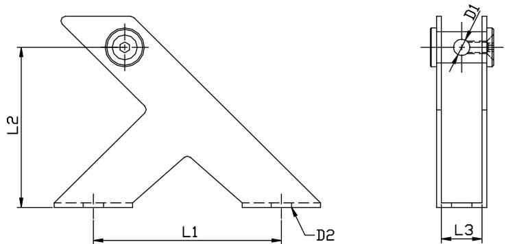
Use max. M5 thread terminals for 3 mm wire
