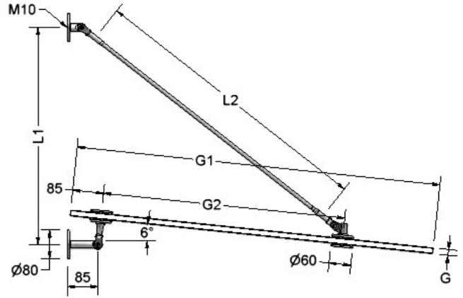
**Blue Wave's Glass Roof fittings are made from AISI 316!**
