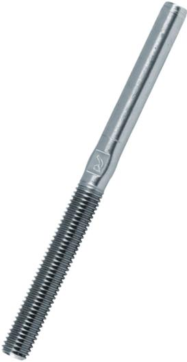
The wide range of threaded Blue Wave terminals are engraved with wire size and swage depth making them easy to use when pressing or swaging them onto the wire. The terminals are available with left handed or right handed threads, and also, on request, with split pin hole (see details below on this page), or UNF thread! Threaded terminals are used to put tension on a wire, either with the help of nuts and washers or as part of a rigging screw.
